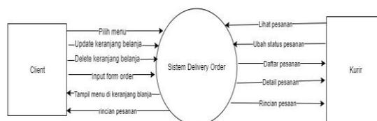
Gambar 5. Data flow diagram level 0.
